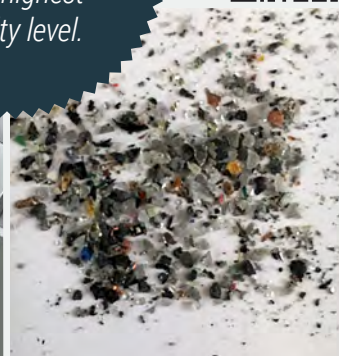
This photo presents the magnified result of destroying a memory hard disk.
